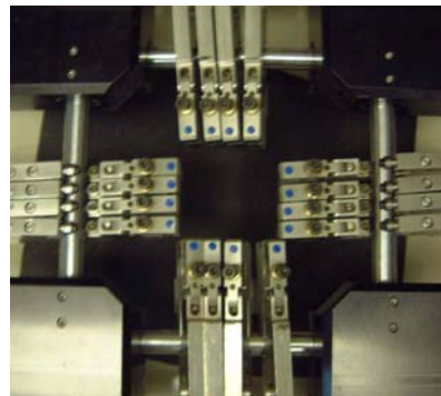
Fig. 4 Chuck for the biaxial tension test device
